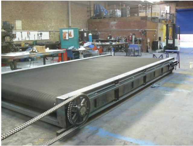
Figur 26 Kedjedrivnet rullband (Central Conveyors Ltd, Odat)
